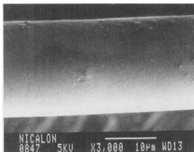
FIGURE 9 3000X SEM photo of a single Nicalon fiber.
